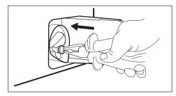
11. Replace the emergency emptying cap into the filter cover and fix it firmly.
